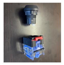
Once the switch is apart you can now use a screwdriver to pop the blue tabs off the bottom of the switch. Becarful not to snap the tabs off.
